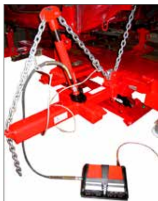
Down pull with pulley
